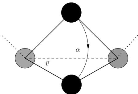
Figure 2.6: Rotation update, which rotates a single monomer by random angle  $\alpha$  around the axis  $\vec{v}$  defined by the two neighboring monomers. This is a pivot-like update, which itself alone is not ergodic, because the end monomers can not be updated.
