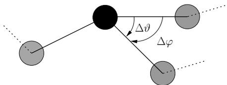
Figure 2.5: Spherical update. One monomer is moved on the surface of the spherical sector with opening angle  $\vartheta_{\max} = 5^\circ$ . The change of the bonding angle is called  $\Delta\vartheta$  and the rotation angle is named  $\Delta\varphi$ . All following monomers are moved by the same difference.
